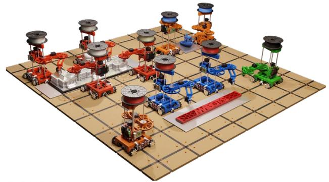
**FIGURE 1:** Demonstration of multi-robot Cooperative 3D printing where multiple jobs are simultaneously printed using multiple robots.
