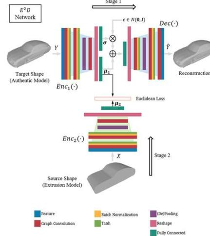
Training module:  $E^2D$  network based on a target embedding variational autoencoder network architecture
