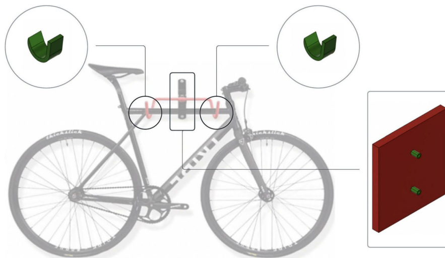
Figure 7. Generative design extra credit module. Context of challenge and starting bike bracket geometry with constraints.
