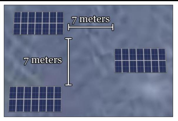
*TIP: To measure Inter-Row Spacing, create an additional solar panel and set it to 7m length. You can then use this to measure the distance between two solar panels.*
