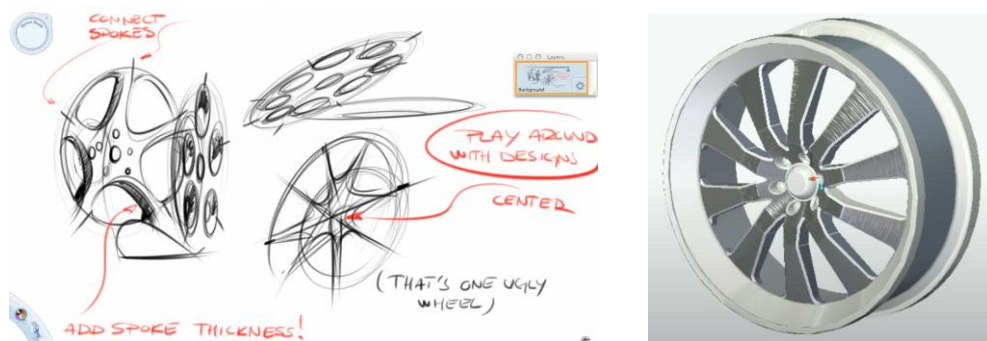
Figure 4. Exploration in car wheel design. Left , Designers often start by sketching various concepts and ideas. They explore different shapes, patterns, and textures that may enhance the performance or aesthetics of the wheels. Right , Designers translate their conceptual sketches into digital models using computer-aided design (CAD) software, where they can further experiment with different dimensions, materials, and finishes.
